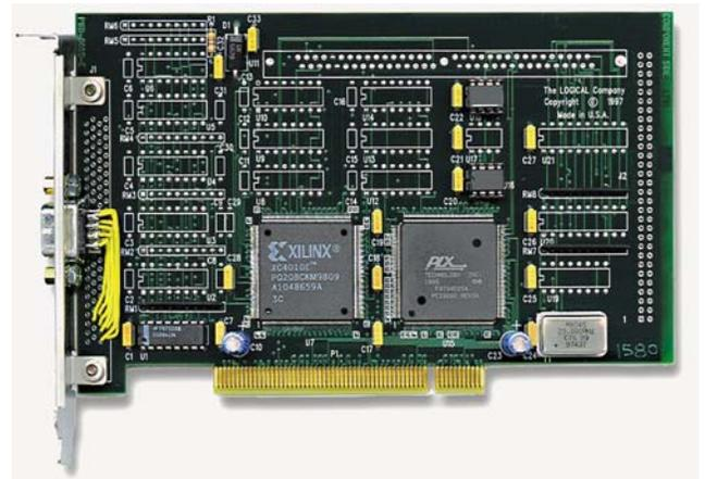
The TMI-2001 is a PCI local bus controller with two independent program-controlled timers. Each timer can be programmed to generate a PCI local bus interrupt at the completion of the selected time interval.
