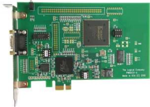
The TME-2001 is a PCIexpress (PCIe) local bus controller designed to replace Logical's TMI-2001 PCI controller for use in newer platforms with a PCIe bus. Like the TMI-2001, the TME-2001 has two independent program-controlled timers. Each timer can be programmed to generate a PCIe local bus interrupt at the completion of the selected time interval.
