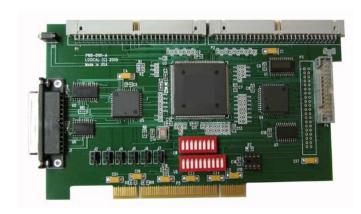
The DQP-3100 PCI-based option module works with Logical's NuVAX 3000 and 3100 systems to allow users to migrate from a Qbus system to a PCI-based system while maintaining their investment in software and user equipment.
